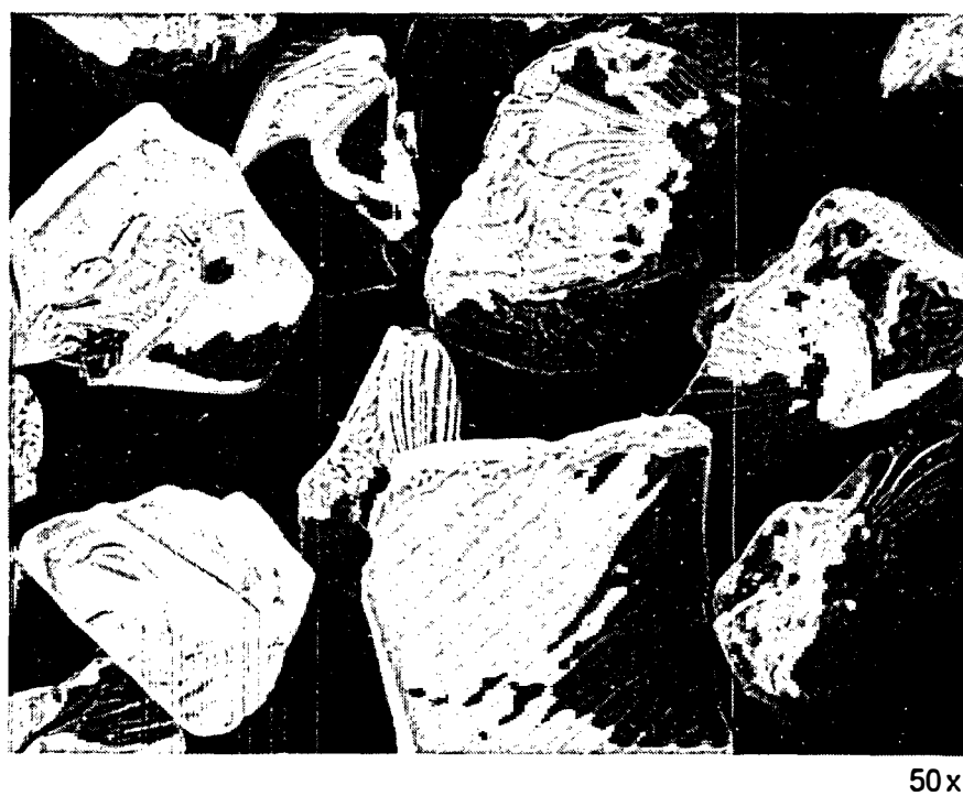
Figure 29. SEM photomicrograph of unirradiated Epicor, Inc. phenolic cation resin at 50 magnification.
